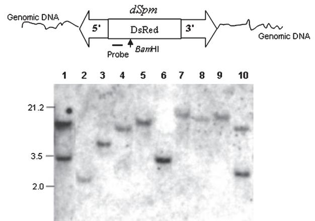
**Figure 3.** Southern hybridization analysis on putative stable insertion lines. Genomic DNA from T<sub>3</sub> transposants was digested with *Bam*HI, and the blots were probed with the *Discosoma sp.* Red Fluorescence Protein (*DsRed*) gene. The transposed defective suppressor mutator (*dSpm*) element should give a band of more than 2 kb. Lane 1, T<sub>1</sub> parental line; lanes 2–10, putative stable transposants.
