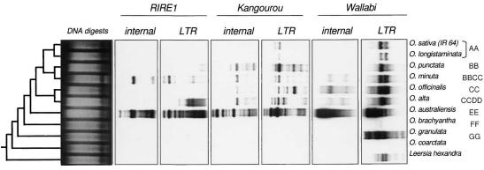
**Figure 4.** Southern hybridization of the three retrotransposons, *RIRE1*, *Kangourou*, and *Wallabi* on total genomic DNA of *Oryza* species digested with Rsal. The phylogenetic tree given on the figure is extrapolated from Ge et al. (1999). The direction of migration is from *left* to *right*.
